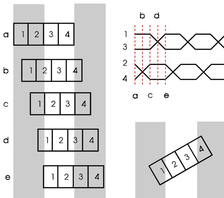
Figure 0-9 Four element photodetector and printed lines
