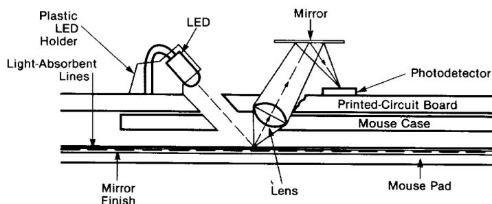
Figure 0-8 Internal mechanical structure of an optical mouse system
