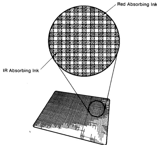
Figure 0-6 Optical mouse pad showing ink lines
