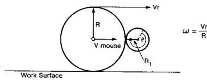
Figure 0-2 Ball and Shaft
