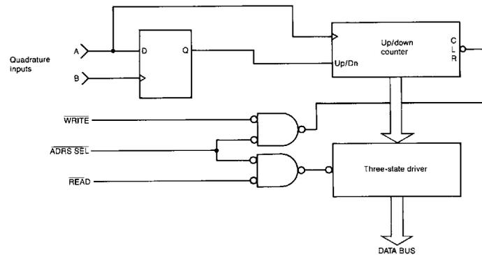
Figure 0-11 Basic quadrature decoder and position counter
