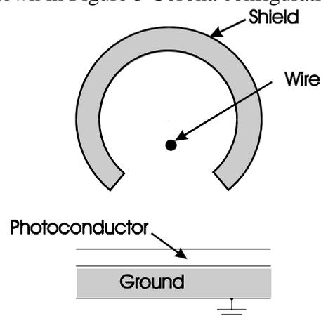
Figure 3 Corona configuration-Corotron
