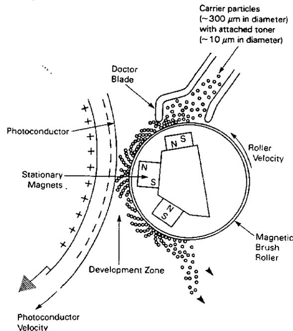
Figure 8 A dual component magnetic brush developer
