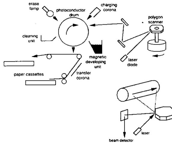
Figure 1: Laser printer printing mechanism
