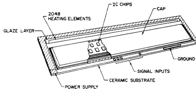
Figure 6 Line thermal printhead with integrated electronic packaging.
