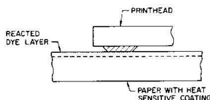
Figure 5 Direct printing on heat sensitive paper.
