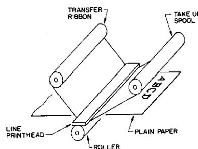
Figure 2 Arrangement for thermal transfer printing using a line printhead, transfer ribbon and plain paper.
