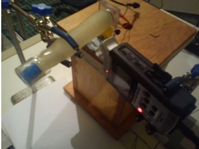
Fig. 3. A photograph of the experimental setup showing a fabricated 22-tube vocal tract model incident with a driving loudspeaker and audio recorder.
